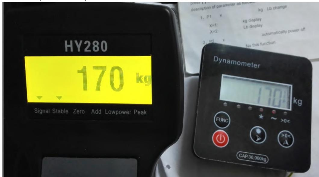
Note: the frequency of both must be set the same, as shown below: 注意：两者的频率必须设置相同，见下图：
