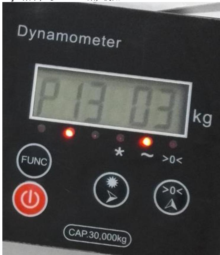
Press [\*] button to exit the frequency setting function and then press the [FUNC] key to return to the weighing state. 按[\*]号键，退出频率设置功能，再按[FUNC]键返回到称重状态。
