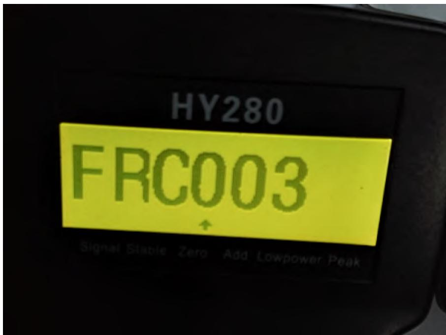
Set the wireless frequency, for example 003# 设置无线频率，例如：003#
